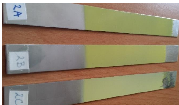
Figure 10 Sample 2, 2A is reference tile, 2B is tile after 30 days under UV light (304 nm) and 2C is a tile after 30 days under second UV light (254 nm)
