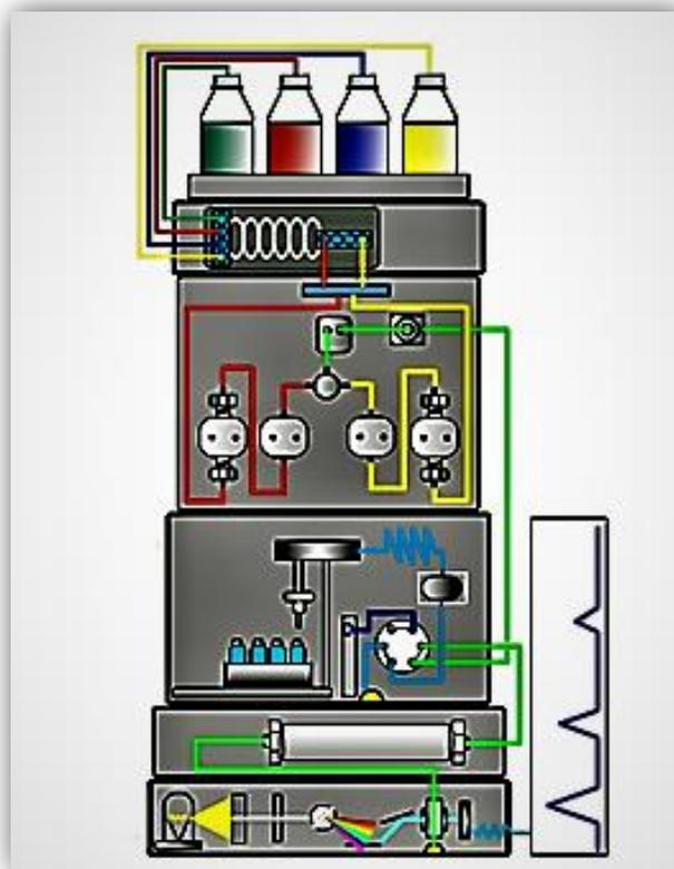
Slika 12. Shema HPLC-a (Tekućinska kromatografija visoke djelotvornosti). Dostupno sa: [https://www.chromacademy.com/HPLC-Operation-part-2.html?tpm=1\\_1](https://www.chromacademy.com/HPLC-Operation-part-2.html?tpm=1_1); pristupljeno: 14.12.2018.
