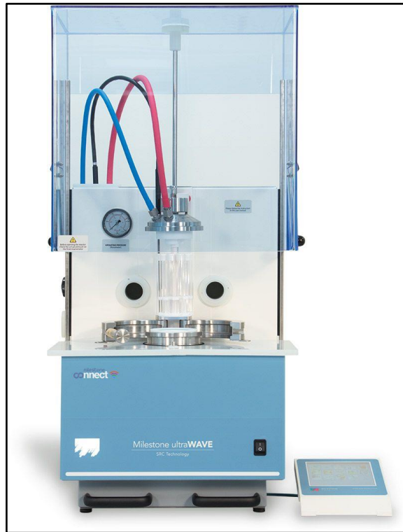
Slika 7. Uređaj za mikrovalnu digestiju - Milestone Srl, Italija (preuzeto s: https://www.milestonesrl.com/products/microwave-digestion/ultrawave )
